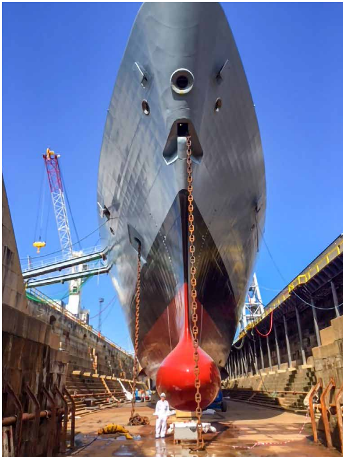
The BAE Systems Platform Manager standing next to the bow dome sonar
