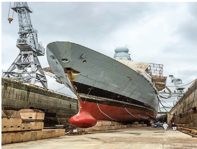
HMS DARING in dry dock, preparing to paint the hull. The white lines are divers' guidelines to key underwater fixtures and fittings that require maintenance whilst submerged.
